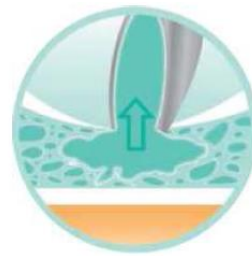
Fig.4. When the sharp point finally penetrates the layer the active component (disinfectant liquid) squirts out by elastic energy restitution.
